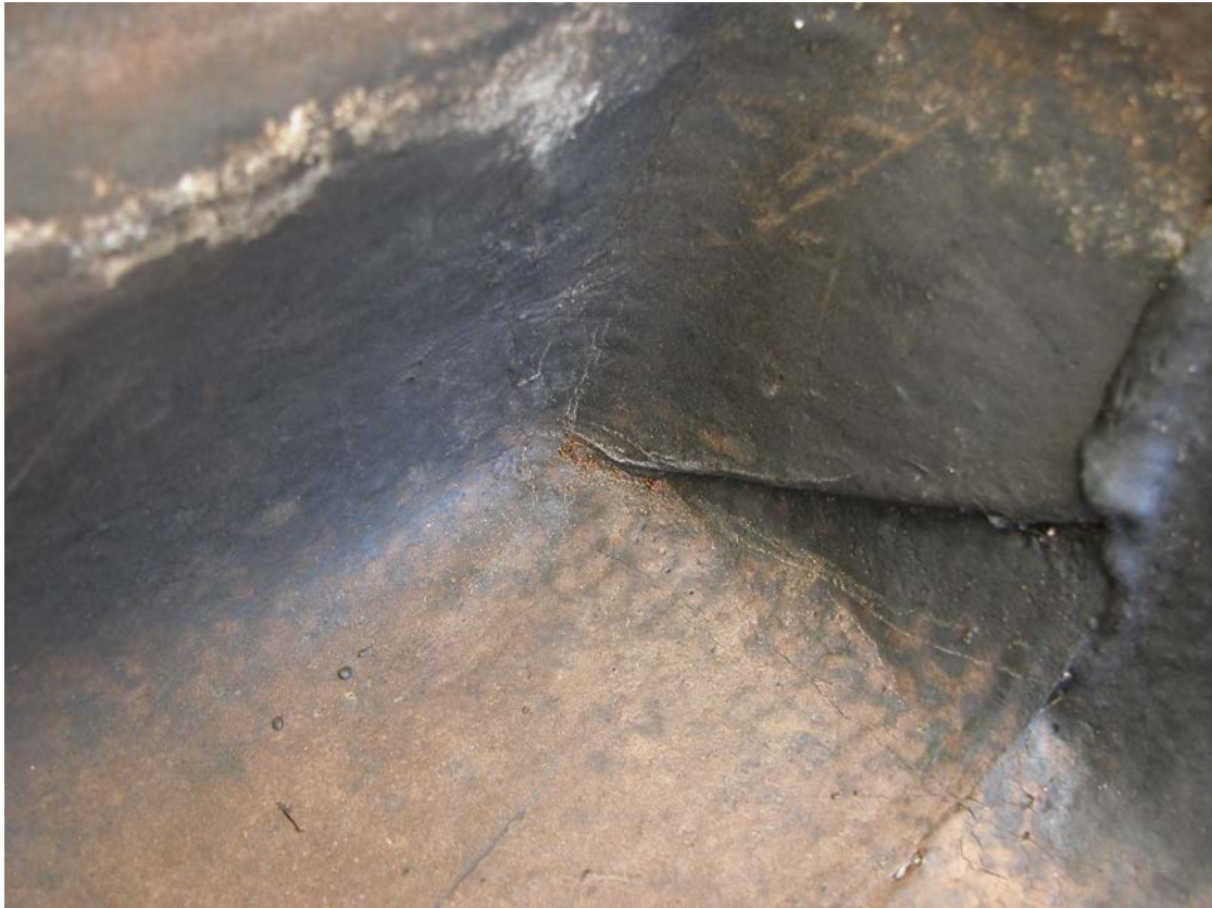
Figure 3: Sheet surface with wall corner joint
